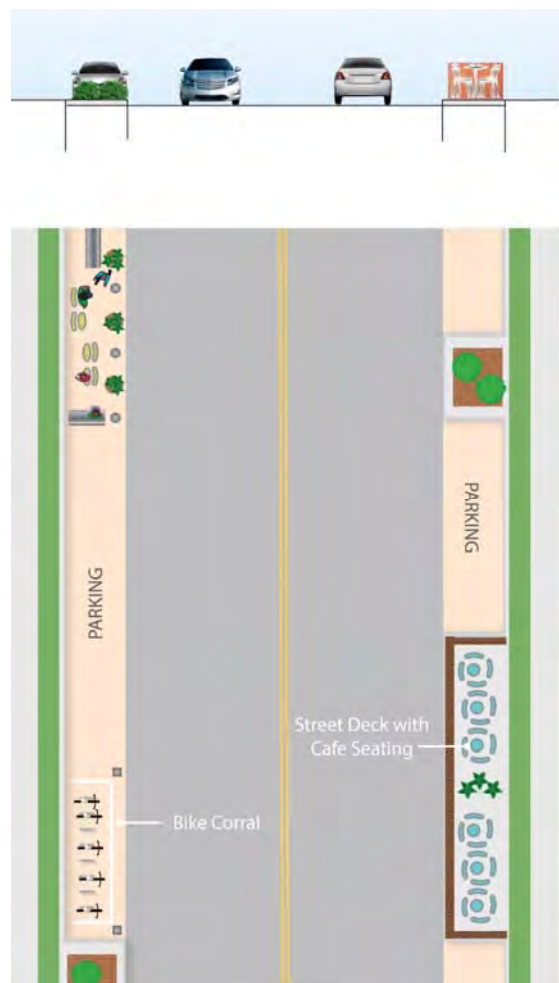
FIGURE 26 - RECOMMENDED KEAWE STREET CROSS-SECTION
