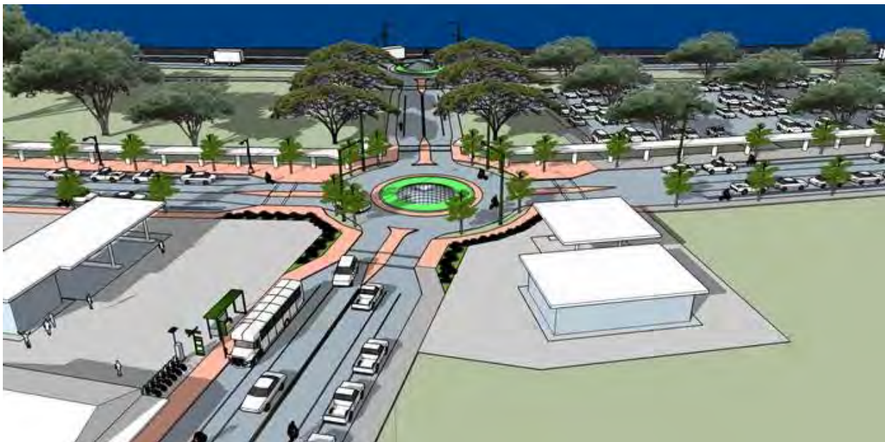
Ponahawai Street extension connecting Kamehameha Avenue and Bayfront Hwy with two roundabouts and covered walkways serving as gateway features.
