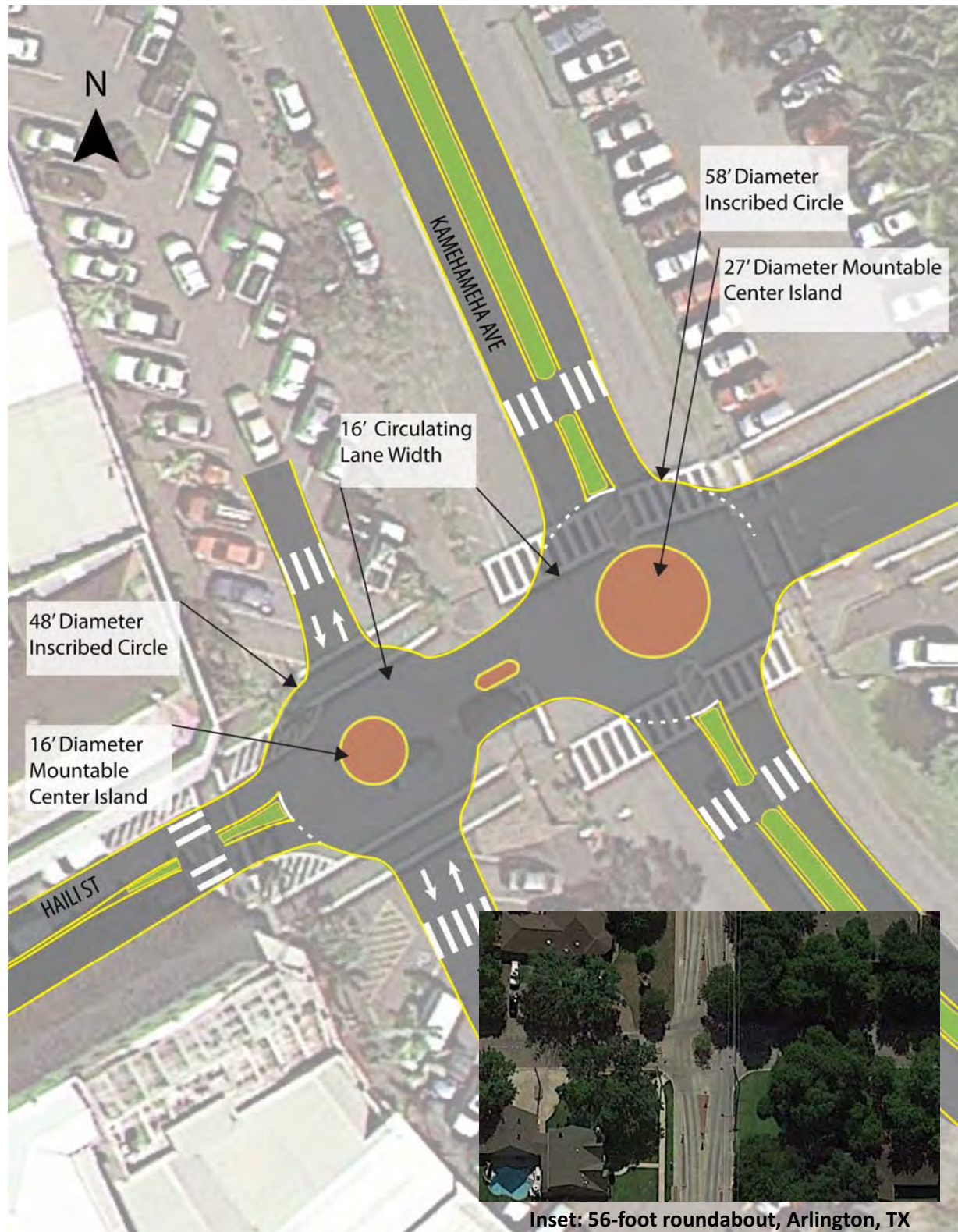
FIGURE 17 – DOUBLE MINI SINGLE-LANE ROUNDABOUT - HAILI STREET AT KAMEHAMEHA AVENUE AND AT FRONTAGE ROAD
