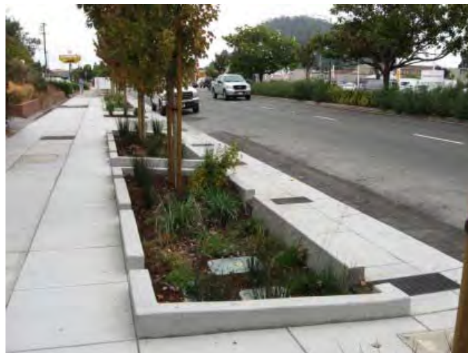
Example of an urban Green Street design using a continuous bioswale planter with drain inlets along the sidewalk and parking lane. (Portland, OR).
