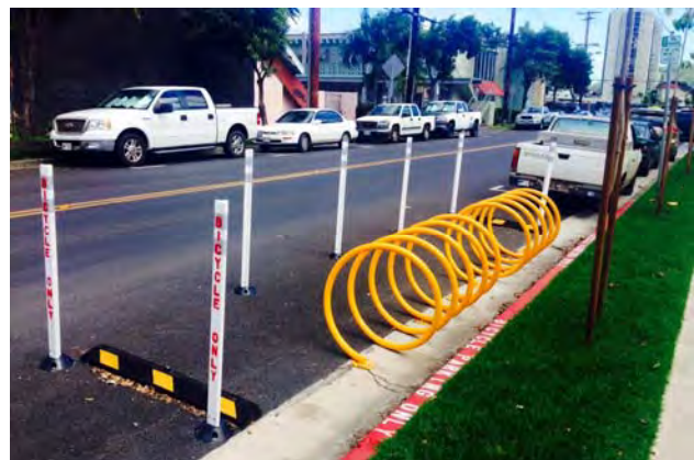
Left: Conceptual bike corral on Keawe Street. Right: Bike corral in Kailua, O'ahu with road and parking buffers along three sides and fixed bike rack within.
