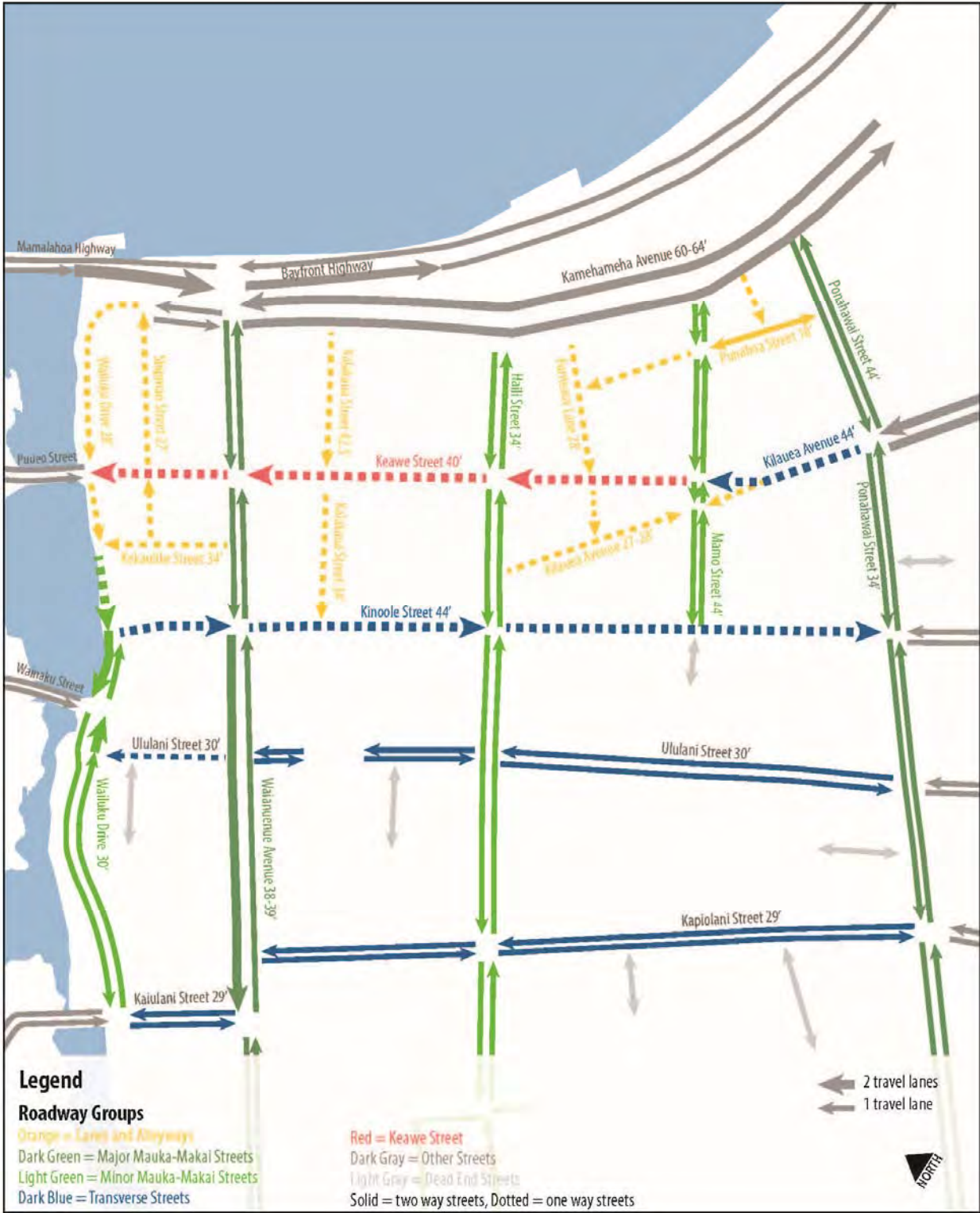
FIGURE 23 - EXISTING PAVED CROSS-SECTION WIDTH
